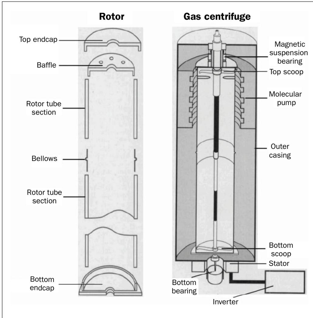
**Figure 3.2.** Basic gas centrifuge design
