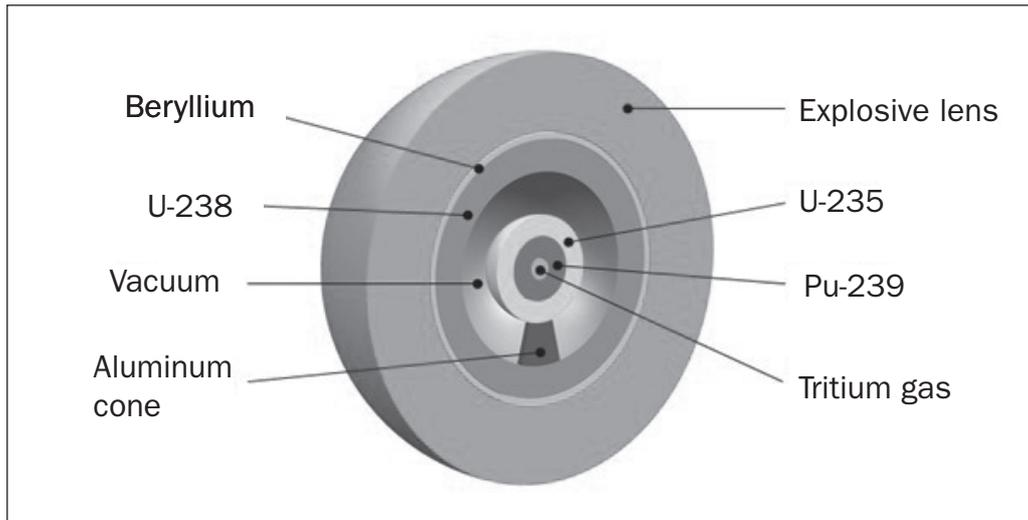
**Figure 3.1.** Basic components of a nuclear core
